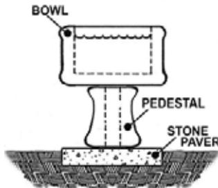
These assembly instructions are generic and based on the principal of re-circulation using a small submersible pump. Although the fountain drawn in Figure 1 may not appear similar in style and individual components may vary, the assembly of components, sealing of cavities and plumbing configuration is identical.
