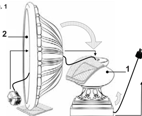
3. With the cord strung through both bowl and pedestal, lift the bowl on top of the pedestal while cautioning not to pinch the pumps power cord between both bowl and pedestal. Do this by removing the slack on the power cord. Once in place level the bowl using a beam level and shims or wobble wedges AG-16 available in clear, black and brown (not included).
