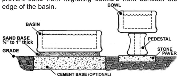
• Pedestals must be placed on a solid surface. Most pedestals are hollow to allow electrical or plumbing to travel through the pedestal. To prevent pedestals from becoming unstable we suggest a solid stone block or paver whenever a pedestal is placed on a soft surface like dirt or grass.
